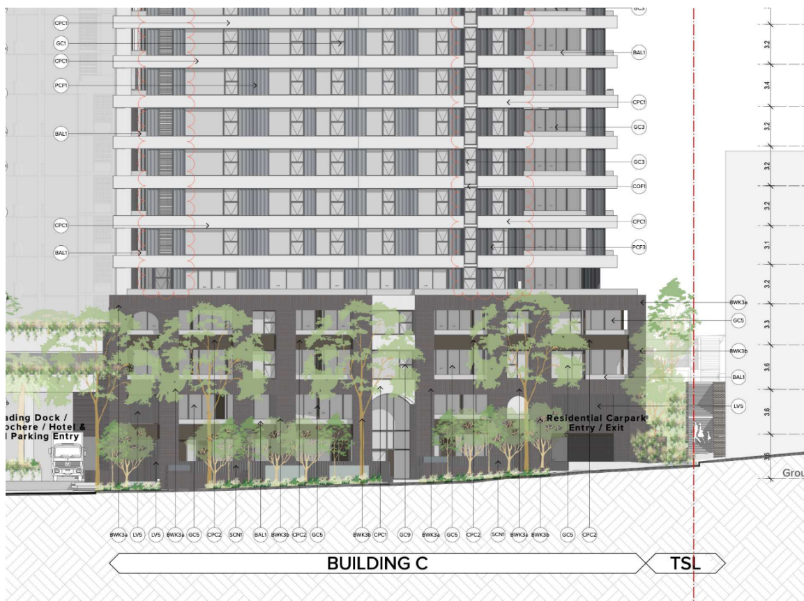
Figure 7: Southern elevation of Building C with elevated ground floor units and 4 storey terrace house appearance.
