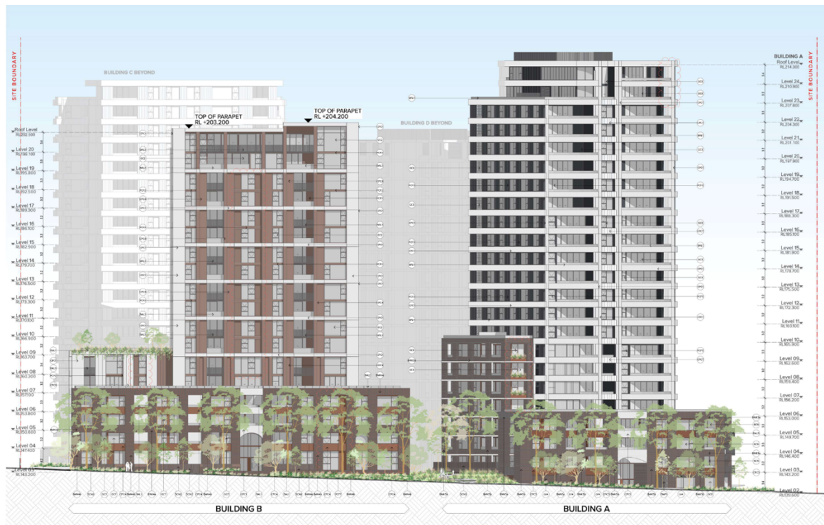
Figure 6: Northern elevation showing façade length of Building B
